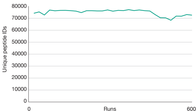
Figure 1: Unique peptide identifications from HeLa QC runs (100 ng) collected throughout a >600-injection series. Samples were analysed on a Bruker timsTOF HT coupled to a nanoElute2 UHPLC system. Raw data were processed in Spectronaut v20.2
