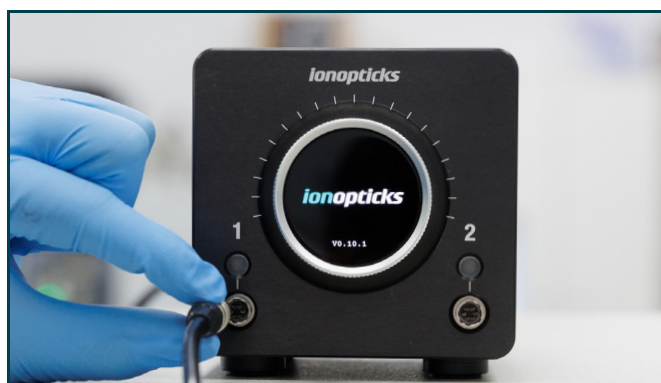
Figure 4. Plugging column heater cable into Channel 1.
