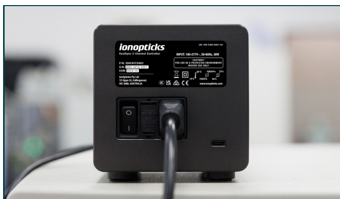
Figure 2. Back panel of the HeatSync™ Controller with power switch in "On" position and power cable connected.
