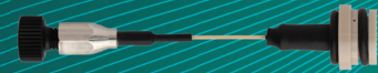
5cm Aurora Series packed emitter column with CaptiveSpray Insert (5cm x 150µm ID, 1.6µm C18) Part No. AUR2-50150C18A-CSI
