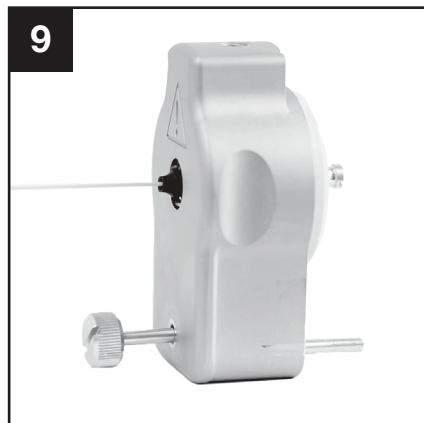
The CSI housing is now ready to connect to your LC-MS system.
