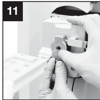
11 Press the CSI Housing with a small amount of pressure and tighten the screw until finger tight.
