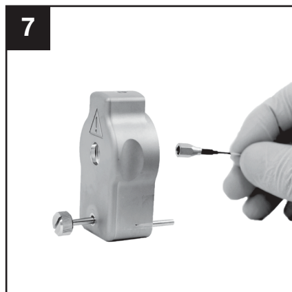
Feed Aurora column with nanoZero® fitting through CSI probe housing.
