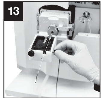
13 Move the column heater in front of the CaptiveSpray source.
