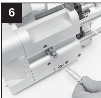
6 Connect the high-voltage cable to the source.
