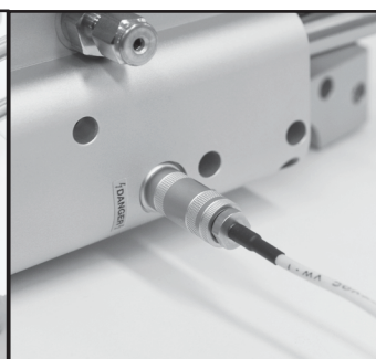
6 Connect the high-voltage cable to the source.
